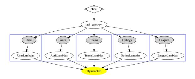
Fig. 1 - High level backend architecture
